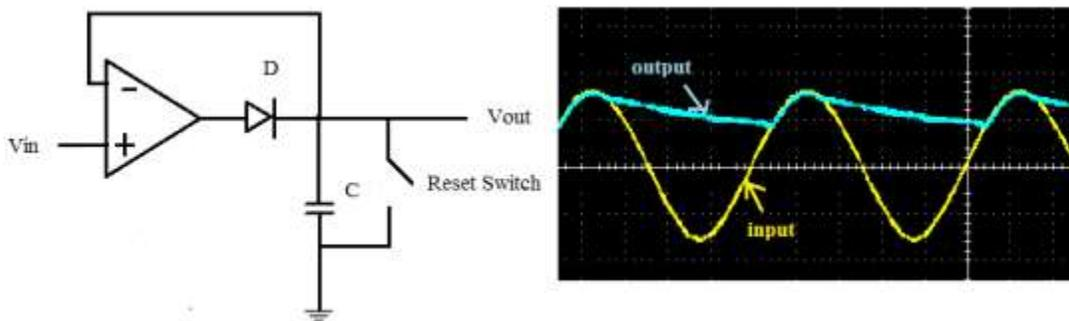
Fig 2. Practical peak detector circuit with input-output waveforms
