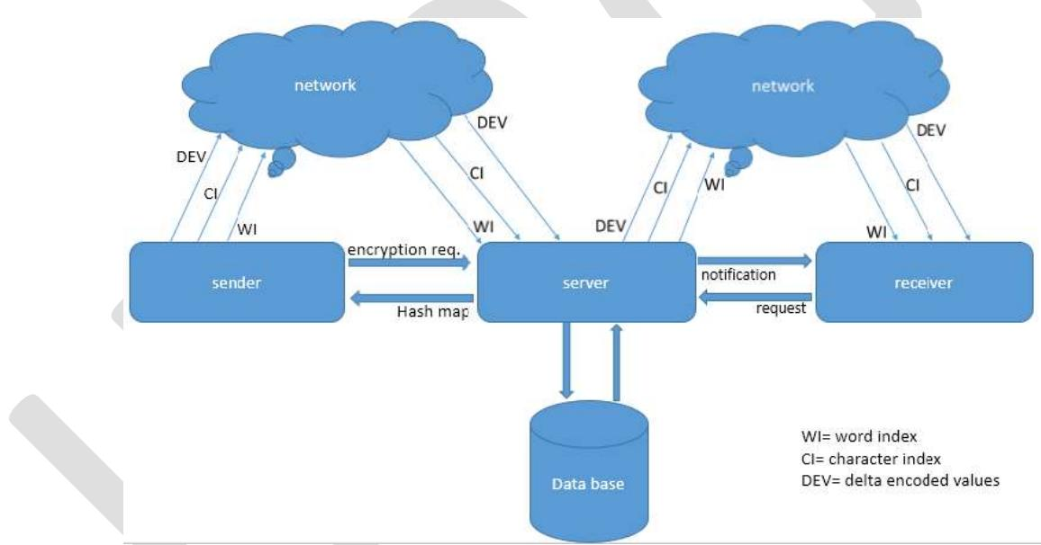
Message entered by user is encrypted at client side and then ciphered text is sent to server and stored on to the server. Server store encrypted message in message data base and then notify appropriate receiver about message. Whenever receiver login into the system and request for the message, server sent ciphered values to the receiver and decryption take place at the receiver end. Then original message will be sent to receivers email address.
