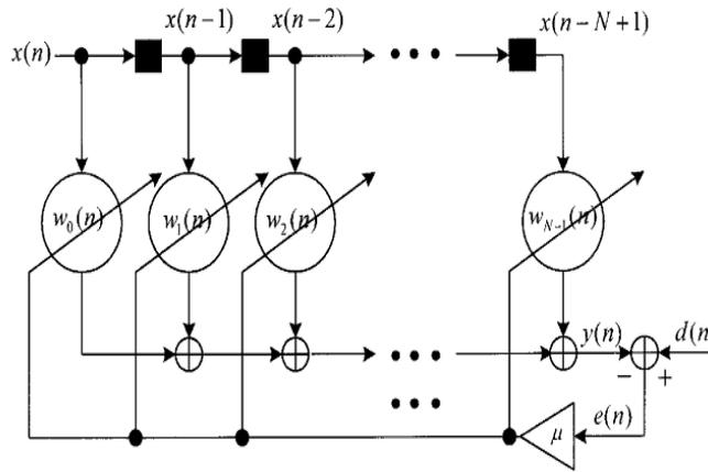
**FIG. 1 LMS ADAPTIVE FILTER**
