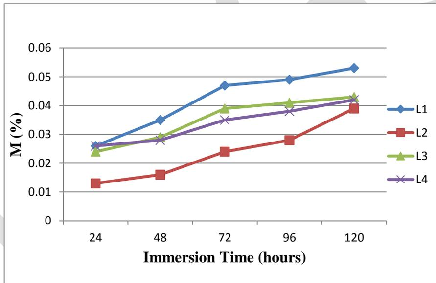
Fig. 11. Water absorption of composites in salt water
