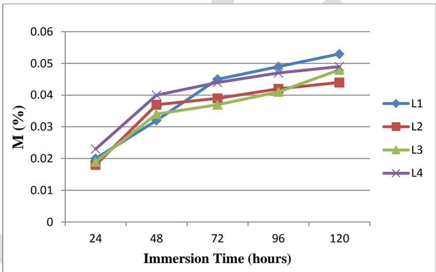
Fig. 9. Water absorption of composites in distilled water
