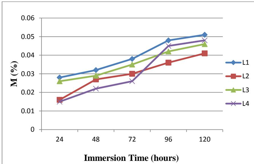
Fig. 10. Water absorption of composites in normal water
